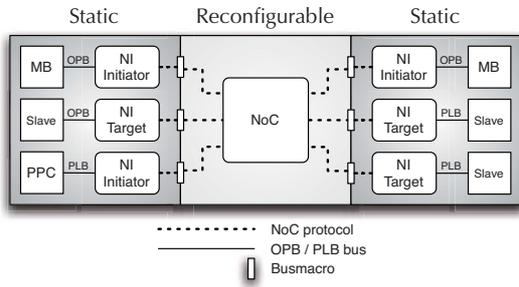
Fig. 2. Interfaces between static and reconfigurable parts
