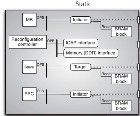
Fig. 3. A static part with a reconfiguration controller
